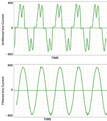
The closed loop control concept also enables the filter to demonstrate excellent performance for achieving target power factor and load balancing.
