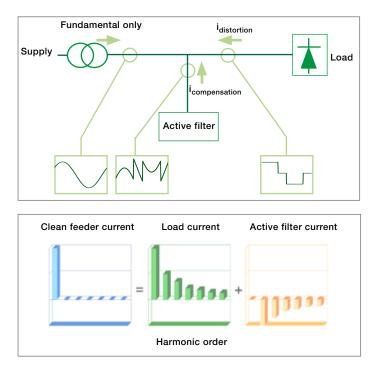
An ABB active filter is a power electronics based electrical equipment that is installed parallel to the polluting loads. It monitors the line current harmonics, as well as the customer requirements programmed by the user. It can then generate for each harmonic frequency a compensation current in perfect phase opposition to the polluting current.
